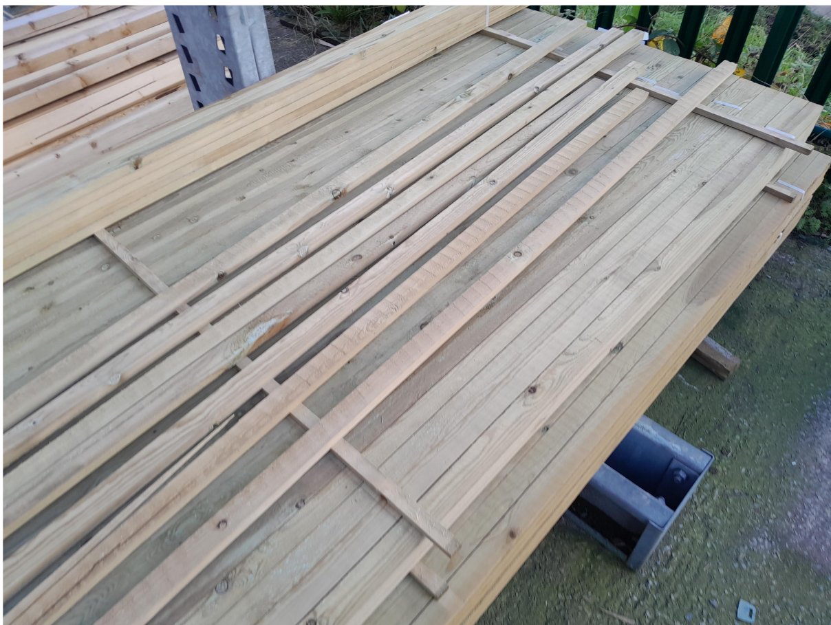
Typical stack of timber with strips that can easily be pulled out
