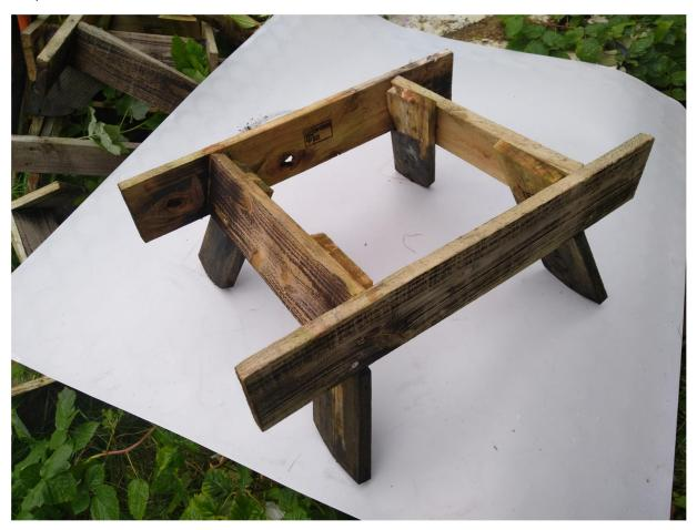
The cross-pieces of wood have a useful length dimension of around 360 to 370mm. This will allow a brood/super/dummy board frame to sit nicely in place off the ground whilst dabbling inside the hive.
